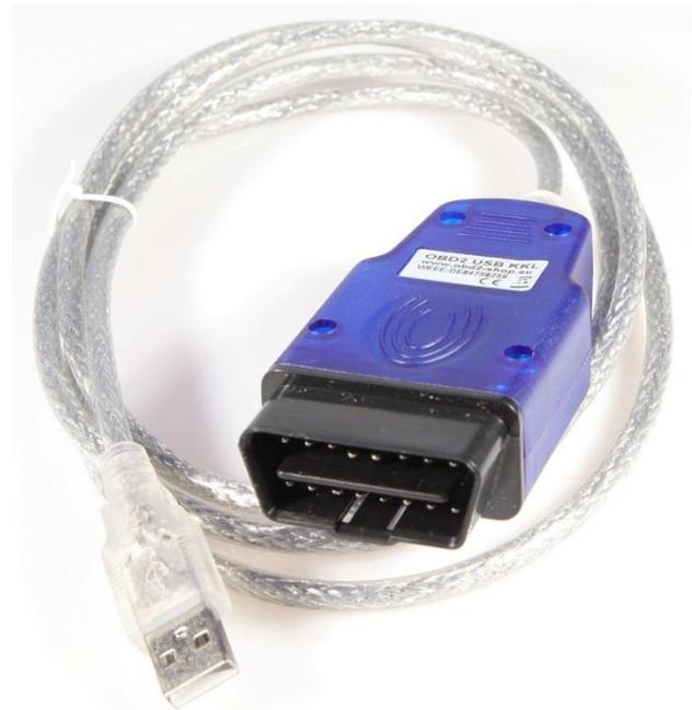
*A typical dongle which plugs into a vehicle's OBD port – in this case the type used by a mechanic to diagnose engine faults. Those used by telematics insurers are very similar, though without the bulky cable. (Source: Wikipedia.org)*
